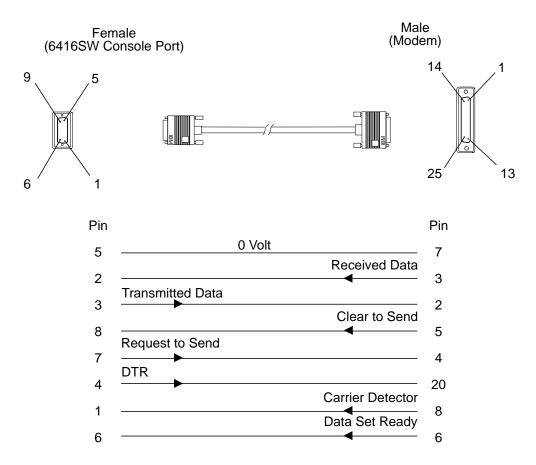
Figure B-5. Pin Assignment: RS-232 Modem Cable
